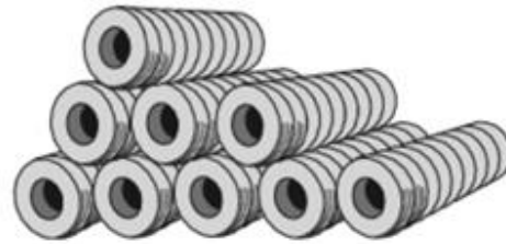
FIGURE A.3.9.4.9(f) On-Floor Storage; On-Tread, Normally Banded.
